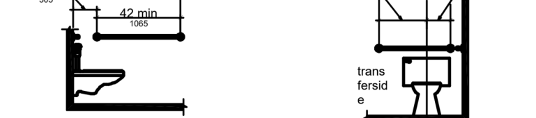
Figure 604.5.1 Side Wall Grab Bar at Water Closets. Figure 604.5.2 Rear Wall Grab Bar at Water Closets
